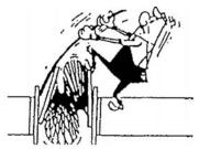
Don't compress or stretch a connector to make it fit. Compression stresses the corrugated element, slackens the braid pressure restrainer, reduces further compressive movement and generally results in early failure. Stretching places excessive stresses on the braid and braid collar and can result in early rupture.
